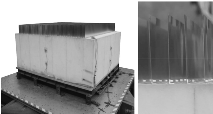
Figure 1.9 Left: Aluminum sheets acting as resonators by means of a shaking table (Bristol Laboratory for Advanced Dynamics Engineering); right: zoom on the sheets (original pictures by Professor Claude Boutin).
